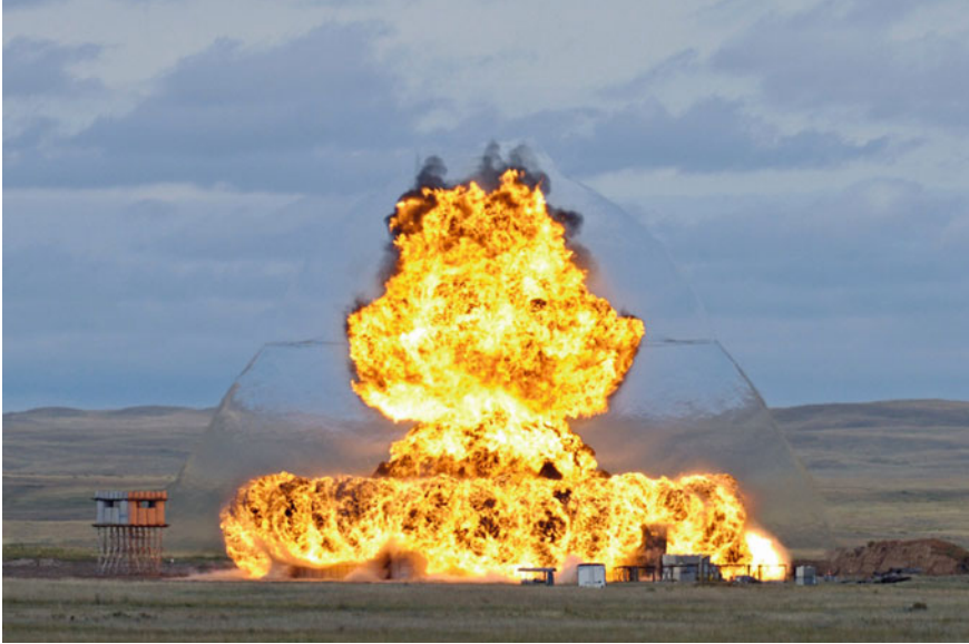
Fig. 1.1 Detonation of a TNT explosive at the ground surface, shock wave is seen expanding radially ahead of the fireball (photograph credits: Defence Research and Development Canada © Her Majesty the Queen in Right of Canada, as represented by the Minister of National Defence, 2015)
