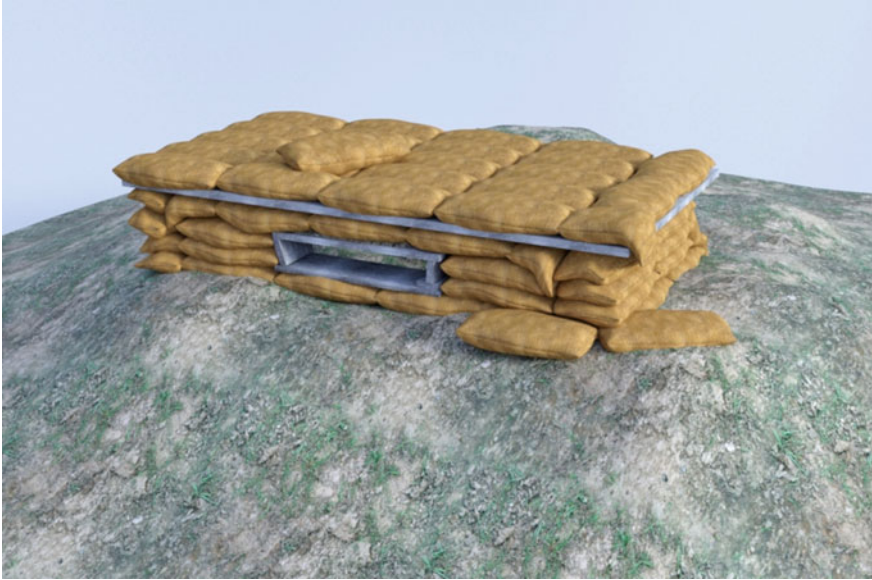
Fig. 5.1 Artistic impression of the bunker built using sand bags
