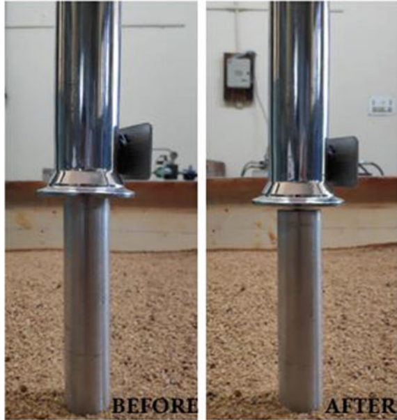
Fig. 8.5 Photograph of the scaled pile model before and after impact of shock wave (shot-1)
