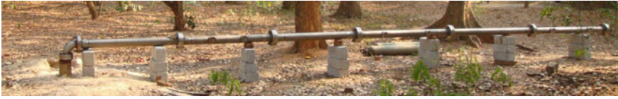
Fig. 8.6 A photograph of fully assembled shock tube connected to the borewell
