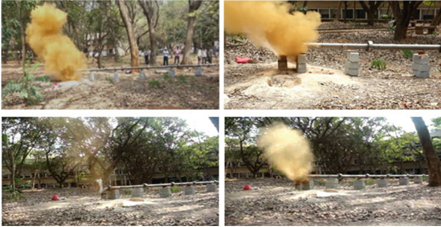
Fig. 8.7 A series of shock waves applied into the borewell (clockwise from top left: shot-1, shot-2, shot-3 and shot-4)
