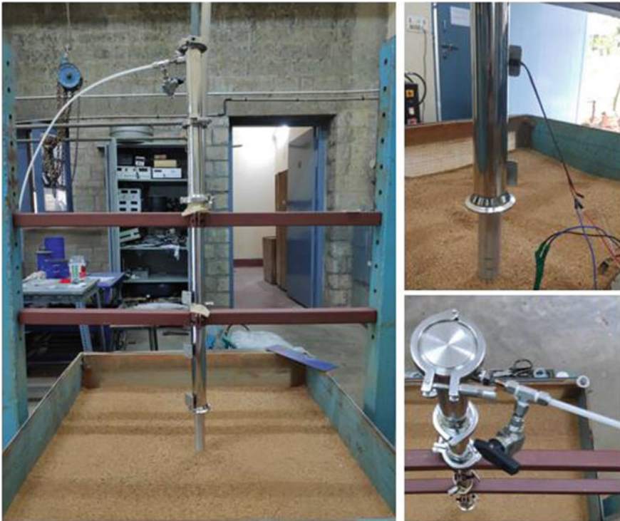
Fig. 8.4 Small-scale vertical shock tube facility for pile driving, left: complete assembly of the setup; top right: instrumentation; bottom right: compressed nitrogen is injected into the driver section
